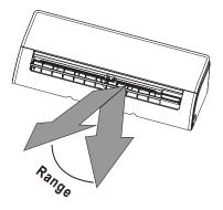
**NOTE:** Do not move louver by hand. This will cause the louver to become out of sync. If this occurs, turn off the unit and unplug it for a few seconds, then restart the unit. This will reset the louver.
