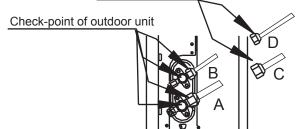
A: Low pressure stop valve B: High pressure stop valve C& D: Indoor unit flare nuts
